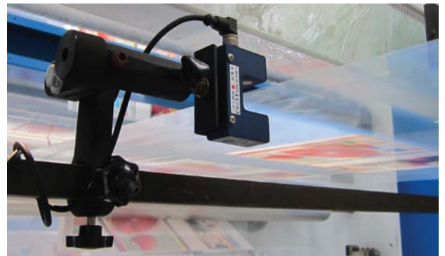
Ultrasonic Sensor DU-1 is used on a Printing Machine
