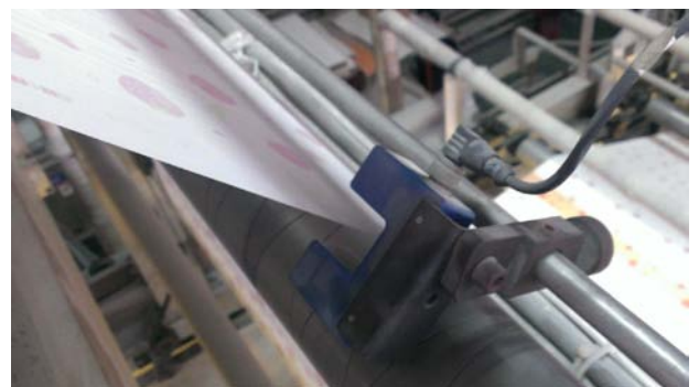
Ultrasonic Sensor DU-1 is used in high dust environment.
